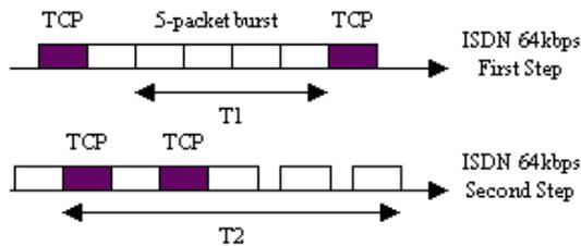
**Figure 8. ISDN bandwidth sharing in presence of TCP competing traffic**
