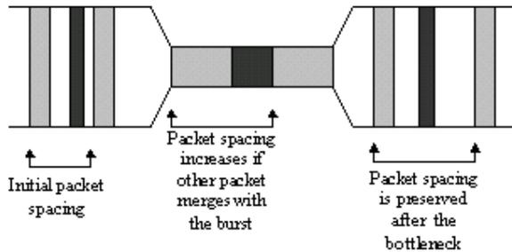
Figure 2. Packet burst sent in the second step
