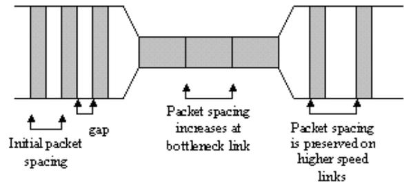
Figure 1. First step: packet burst through a bottleneck link
