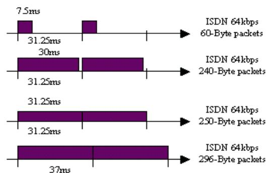
Figure 7. Importance of packet size in bandwidth estimations
