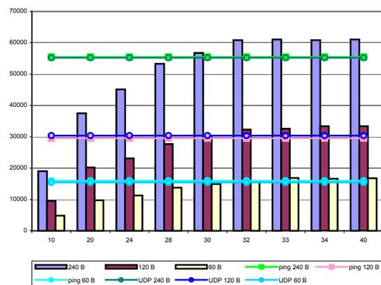
Figure 6. Bandwidth estimation using ICMP or UDP packets in the burst in absence of competing traffic vs. sending UDP traffic only
